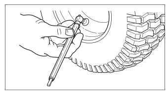
Figure 14. Checking Tire Pressure
